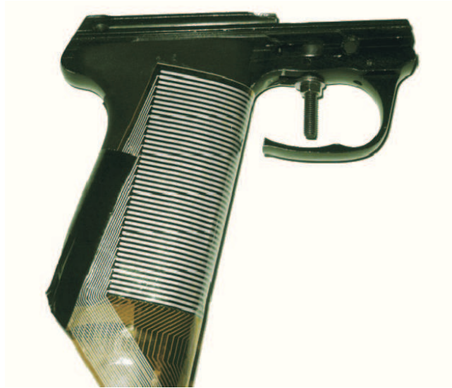
Figure 2.4: SmartGun prototype, with a piezo-resistive pressure sensor on the grip.
